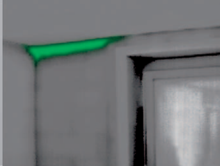
Presentation of surface moisture for detecting mould risk spots
